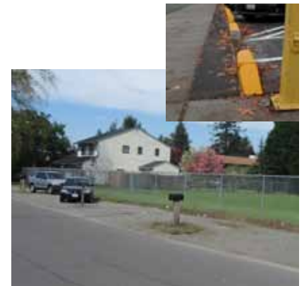
Recommendations 1 and 3 suggest using car stops to designate angle in parking and create a pedestrian walk way between cars and fence.
